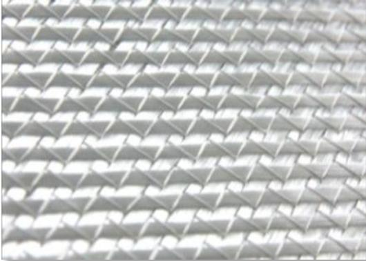
**ARMATON multiaxial fabric** is a textile material consisting of one or more layers of glass fibers. The layers are oriented in various directions and stitched with a polyester yarn. ARMATON multiaxial fabrics are manufactured using state-of-the-art equipment from Germany, which guarantees output of high-quality products.
