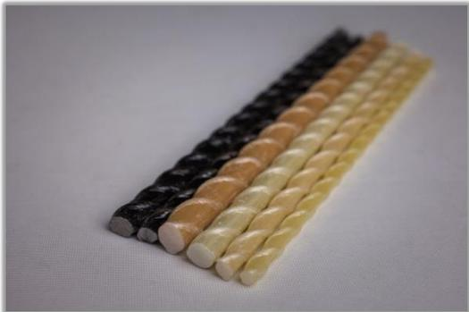
**STEKON fiber-reinforced polymer bar** (composite rebar) refers to rods made of reinforcing fibers impregnated with a polymer thermosetting binding agent and cured, with transversal or helical ribs made on surface of the rods
