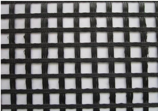
**Neftegaz GRUNTSET geogrids** are glass grids formed by two systems of rovings arranged perpendicular to each other, interknit with a third yarn, a knitting yarn, and impregnated with a polymer compounds.
