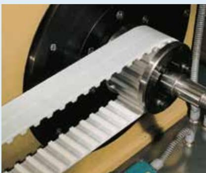
In modern power transmission and handling technology Siegling Proposition timing belts are highly versatile machine components which operate economically, accurately and reliably.
