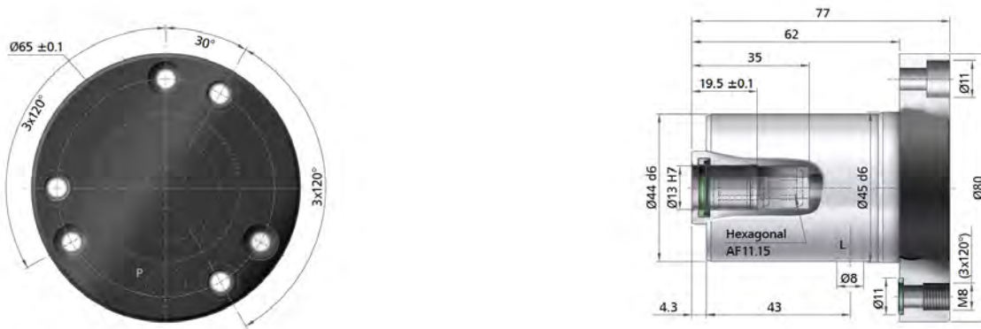
ROTODISK S2-S, Type 10573 – 10,000 rpm / Emulsion, 70 bar / Air, 10 bar
